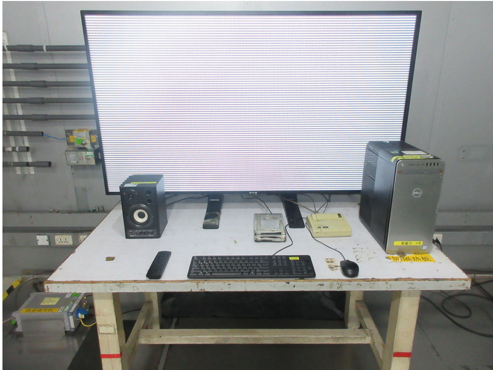
AC Power Line Conducted Emissions
