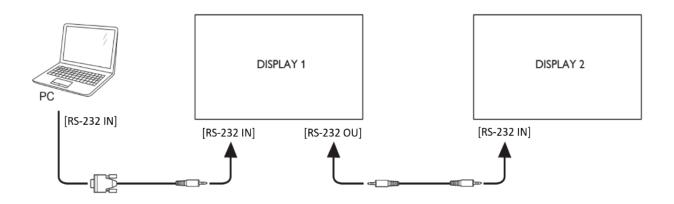
Note: A USB to RS-232 adapter is necessary for computers which do not have a physical serial port.
